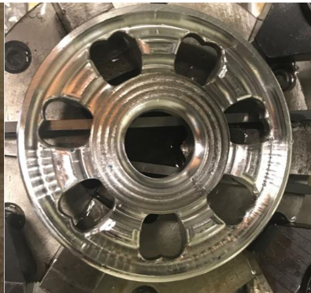
Right: After intense CNC machining
