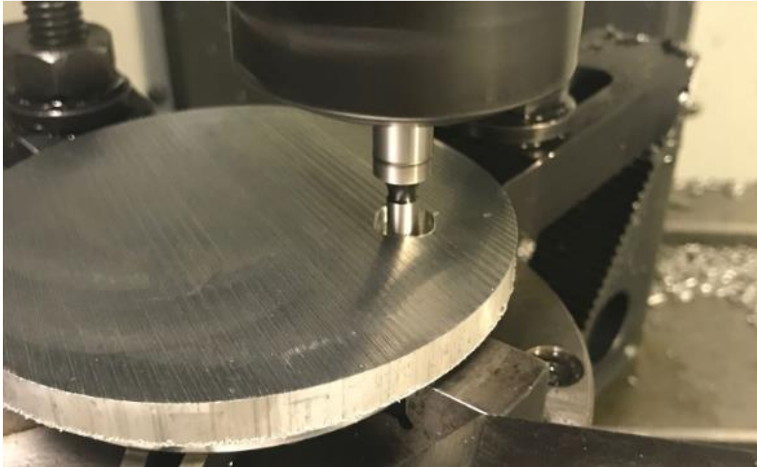
Edge finding the previously machined reference point
